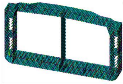
Figure 3. Finite element model.
